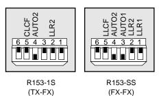
When setting DIP switches<sup>\*</sup>, the UP position is when the lever of the switch is pushed away from the circuit board. The DOWN position is when the lever of the switch is pushed toward the circuit board.
