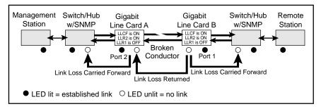
**IMPORTANT:** LLR must not be active on both ends of the same cable. If it is, the link can never be established.
