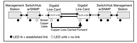
Loss of link at the fiber port is not propagated, as shown below.
